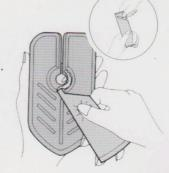
Clip Diverting Collar around pipe and slide a length of sealing strip (rounded edge uppermost) along the slit at rear of collar up to the pipe. This seals the back of the collar.
